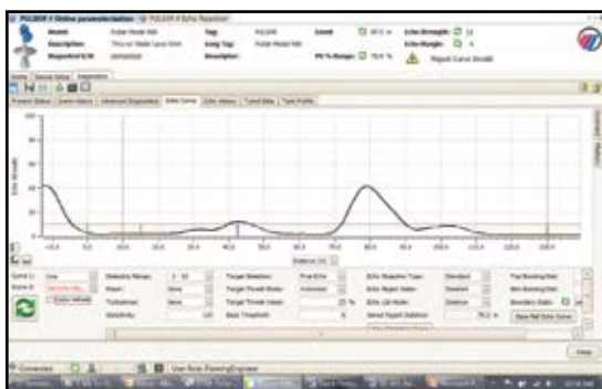
Figure 1. Echo curve (being shown in DTM utilizing PACTware) being shown after having been automatically captured by transmitter.
