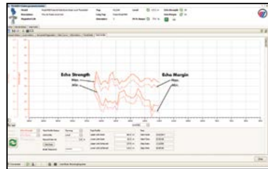
Figure 2. Tank profile graph showing collection of minimum and maximum values for echo strength and echo margin
