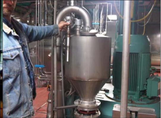
Previously-used single-point capacitance probe
