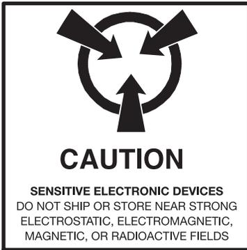
MAGNETROL electronic instruments are manufactured to the highest quality standards. These instruments use electronic components that may be damaged by static electricity present in most work environments.
