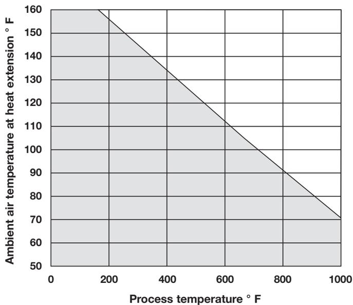
The heat dissipation graph, at left, depicts the maximum temperatures at which the extension can be used effectively.
