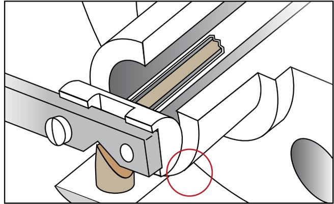
Above: The Torque Tube is susceptible to fatigue failure and accelerated corrosion. Below: The static-pressure-retaining enclosing tube on the E3 Modulevel® is not susceptible to either of these failure effects.
