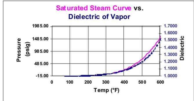
Figure 7. Saturated steam curve vs. dielectric of water vapor
