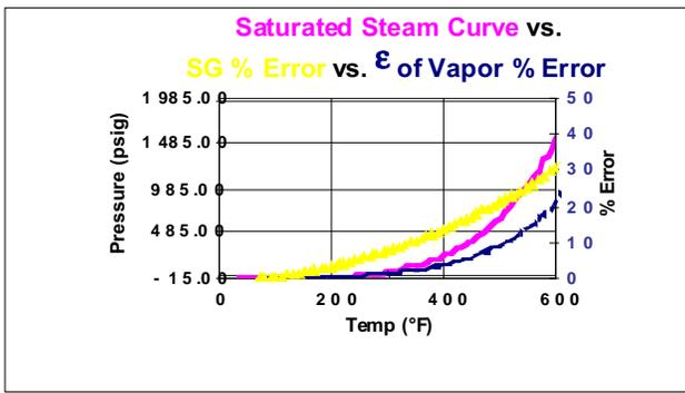
Figure 9. Saturated steam curve showing comparison % error specific gravity vs. % error dielectric of vapor space above liquid.
