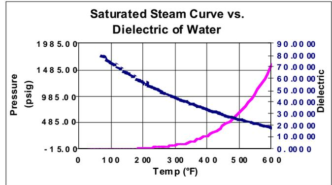
Figure 5. Saturated steam curve vs. dielectric constant of water.
