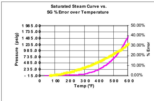
Figure 3. Saturated steam curve vs. % error of specific gravity variation of water.
