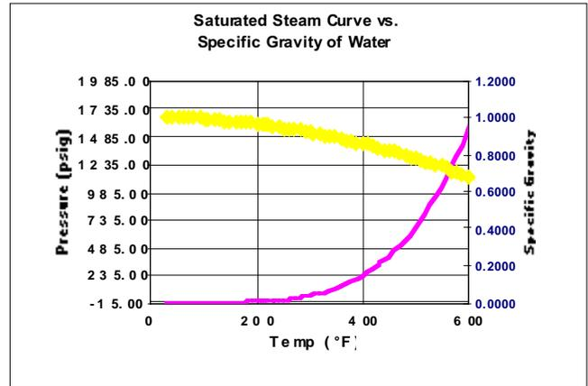
Figure 2. Saturated steam curve vs. specific gravity of water.
