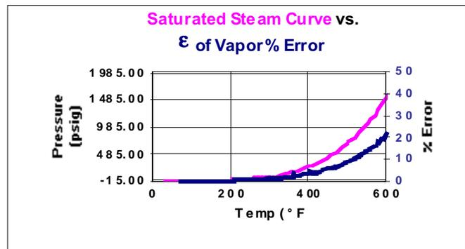
Figure 8. Saturated steam curve vs. % error of the dielectric constant of water vapor.
