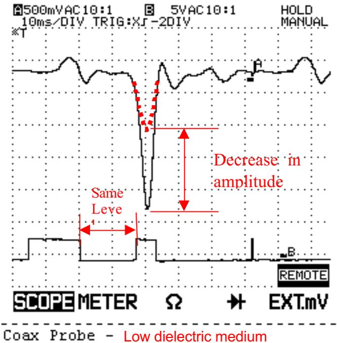
Figure 6. Oscilloscope trace showing reflection amplitude decreasing dielectric constant of liquid yet its point in time (position) remains constant.
