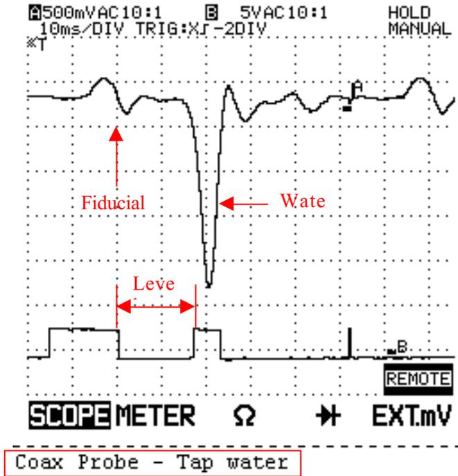
Figure 4. Oscilloscope trace of Guided Wave Radar showing Fiducial (baseline reflection) and strong reflection received from water (high dielectric medium).
