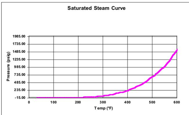
Figure 1. Saturated Steam Curve
