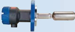
The TUFFY II buoyancy level switch is a float-actuated device designed for horizontal mounting in a tank or vessel through threaded or flanged pipe connections. The compact size allows for installation in small vessels, while its many features provide a variety of application uses. The single switch mechanism is available in SPDT or DPDT forms on units designed for fixed or adjustable, narrow or wide differential and interface service levels.
